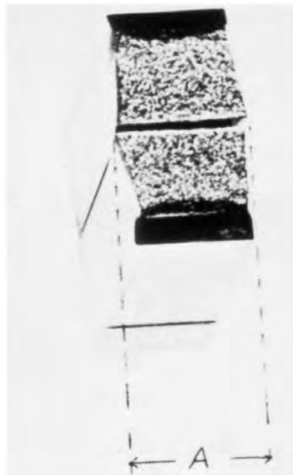
FIG. 15 Halves of Broken Charpy V-Notch Impact Specimen Joined for the Measurement of Lateral Expansion, Dimension A
