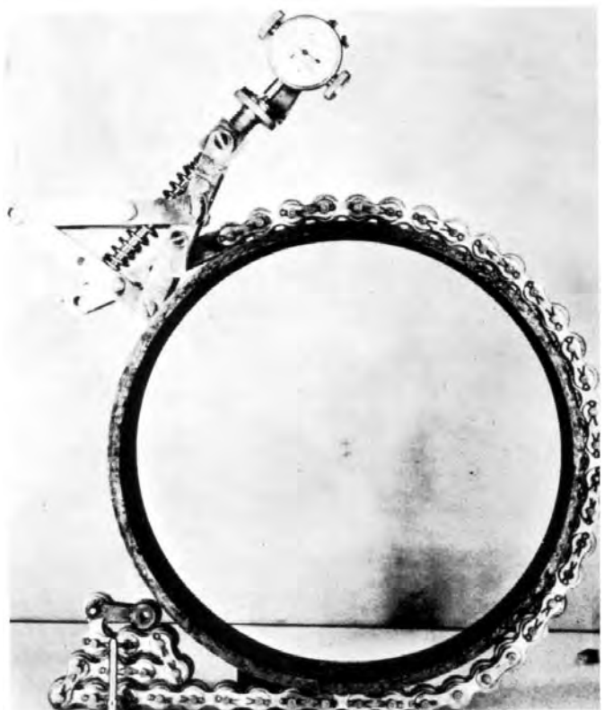
FIG. A2.7 Roller Chain Type Extensometer, Unclamped
